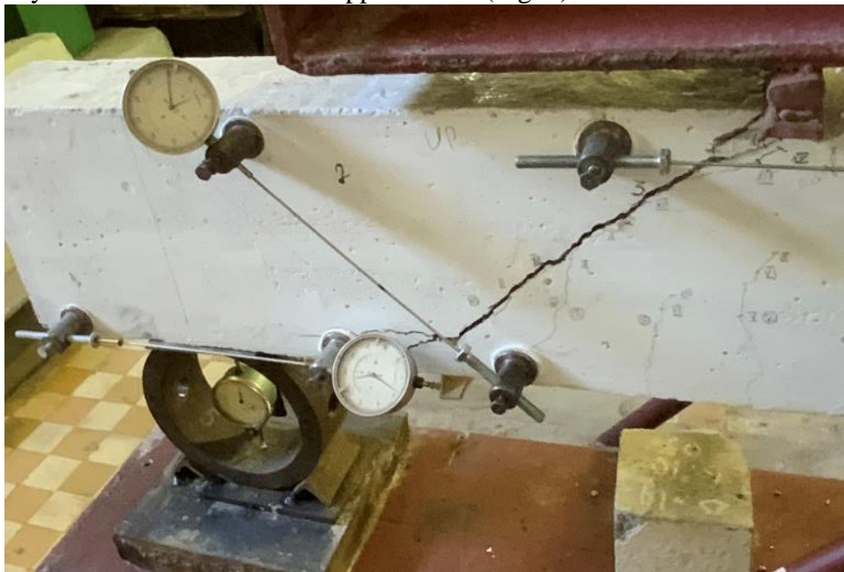
Fig. 3. A crack along the left inclined section
