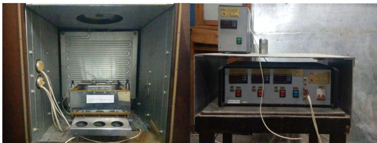
Figure 5. Installation for testing thermal conductivity at a temperature of 10 °C
