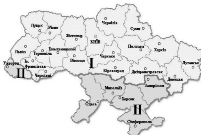
Fig. 5. Schematic map of temperature zones in Ukraine (SCS V.2.6-31: 2016 "Thermal insulation of the building," Appendix B [4])
